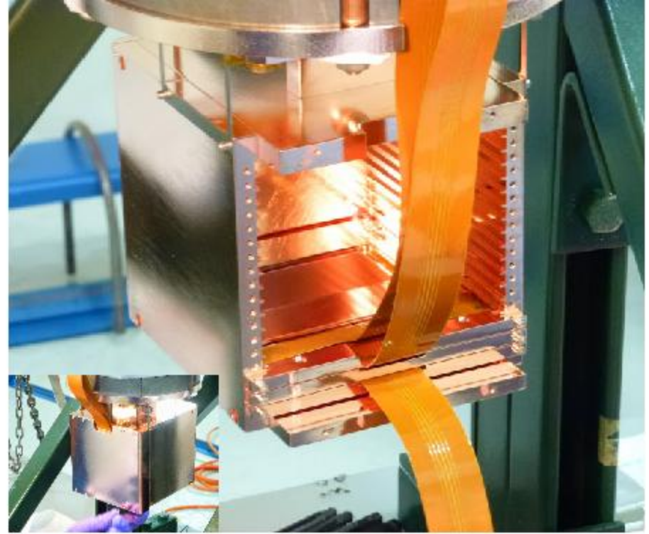
Stack of 18 CCDs (8 sensor prototype shown here)
